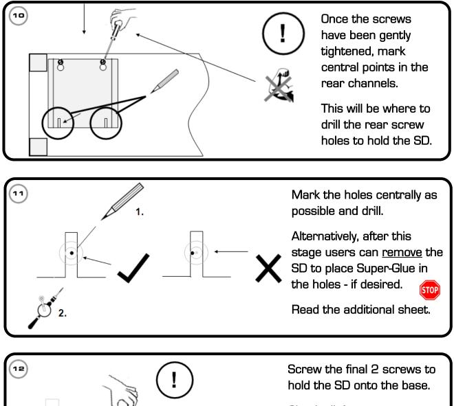
Check all 4 screws are gently tightened especially if Super-Glue is not used.
